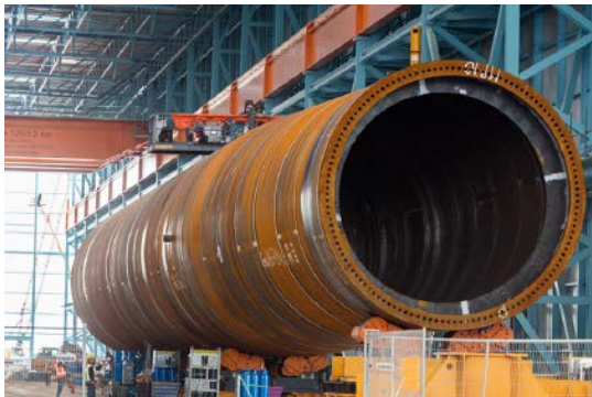
Monopile assembly at Maasvlakte 2
