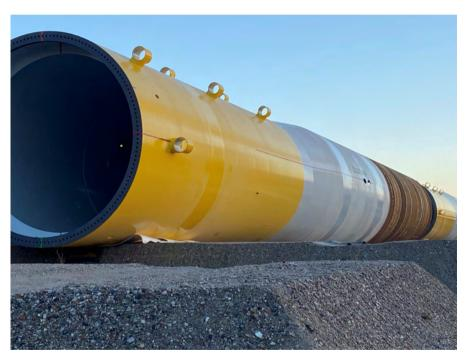
Picture: the diameter of a monopile refers to the diameter at the bottom. Towards the top of the monopile, the diameter reduces to 7.5-8.5 meters using cones to match the diameters of the tower or transition piece
