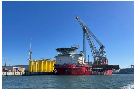
Monopiles and Transition pieces for Dogger Bank A&B
