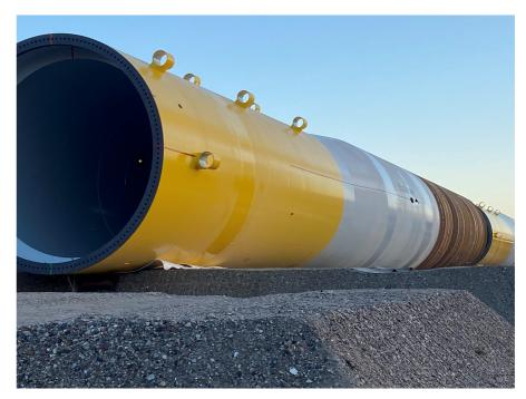
Picture: the diameter of a monopile refers to the diameter at the bottom. Towards the top of the monopile, the diameter reduces to 8 meters through the use of cones to match the diameters of the towers or transition pieces
