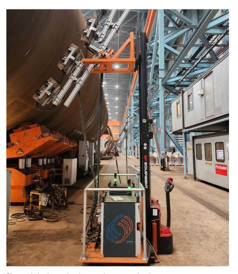
Pictures: induction pre-heating to replace gas pre-heating
