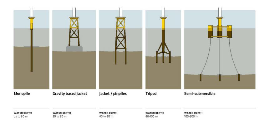
Picture: the range of foundations applied for offshore wind turbines
